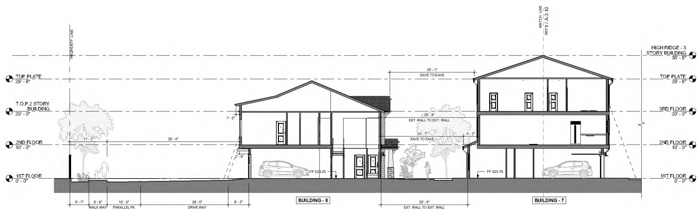
② TYPICAL SITE SECTION FROM S LIVERMORE AVENUE - BLDG. 7 & 8 1/8" = 1'-0"
